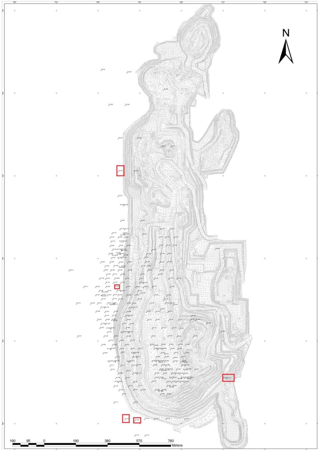
Figure.4 Schematic of the Sadiola main pit indicating locations of boreholes (red boxes) which have been studied in this project.
